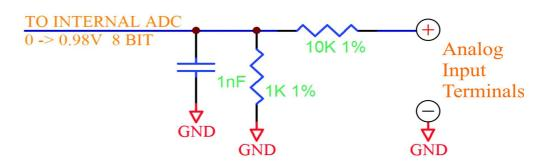
The GSM Commander provides a single 0-10.8V analog input, which can be used to measure incoming voltages from sensor devices or power sources (example: battery banks). Using an appropriate resistor, one can also connect 4-20mA sources to the GSM Commander. (See application note under section 18)
