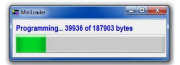
The loader utility will now show this screen, which means the firmware is being updated. The green LED, labeled "STATUS" on the GSM Commander, will start flashing.
