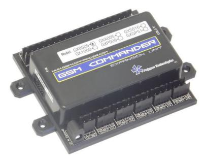
The GSM Commander supports comprehensive expansion by means of the GSM Commander Expansion unit, which provides an additional 5 inputs and 5 outputs similar to the ones found on the GSM Commander itself. A total of 6 Expansion units may be daisy chained to provide a maximum of 30 outputs and 30 inputs\* in addition to those on the GSM Commander itself.
