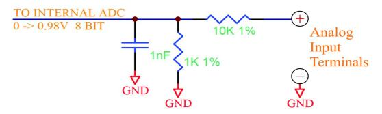
The GSM Commander provides a single 0-10,8V analog input, which can be used to measure incoming voltages from sensor devices. Using an appropriate resistor, one can also connect 4-20mA sources to the GSM Commander. (See application note under section 18)
