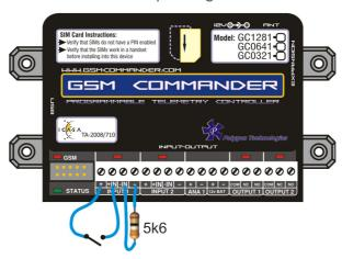
To connect a switch or contact to an input, simply connect the switch between the + and +IN terminals, and a **5k6** resistor between the - and IN- terminals. The reverse is just as suitable, i.e. that you connect a **5k6** resistor between + and +IN and place the switch between - and IN-. This will decrease each input's current consumption (when active) from 25mA to 2mA.
