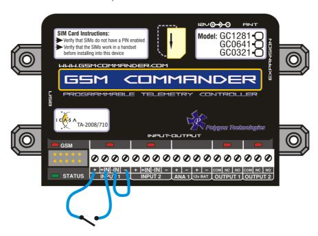
You may need an input to activate when power is supplied from some other unit. A good example will be a burglar alarm that applies power to the wires going to the siren. In such a case, it will be a simple matter of connecting the positive wire to the +IN input, and the negative wire to the -IN input.
