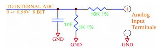
The GSM Commander provides a single 0-10.8V analog input, which can be used to measure incoming voltages from sensor devices or power sources (example: battery banks). Using an appropriate resistor, one can also connect 4-20mA sources to the GSM Commander. (See application note under section 18)
