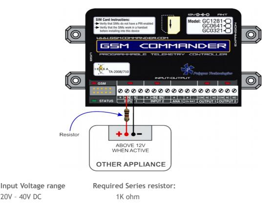
The + and - terminals are connected to the input power supply of the GSM Commander.
