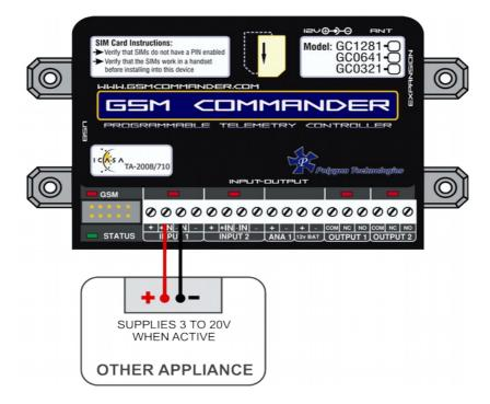
Please keep in mind that these inputs are designed for 3V to 20V operation. If you require to connect a voltage above 20V to these terminals, you should connect a resistor in series with the input, as shown below.
