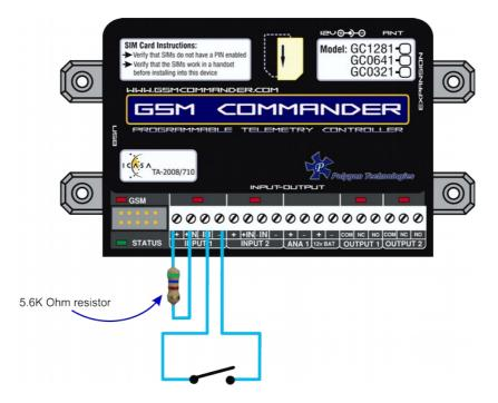
Similarly a **5K6** resistor can be connected to all the inputs of the Expansion Unit(s) to decrease each input's current consumption (when active).
