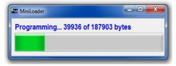
The loader utility will now show this screen, which means the firmware is being updated. The green LED, labelled "**STATUS**" on the GSM Commander, will start flashing.
