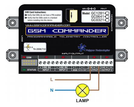
This output can be used to control devices and appliances, and is rated for 8A DC. It may be used to control most types of electrical loads, excluding AC motors above 500W.
