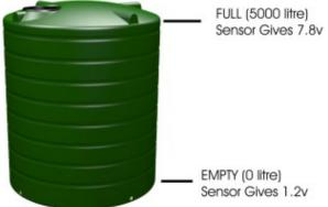
You would thus tell the software that 7.8V should correspond to 5000 litres, and 1.2V should correspond to 0 litres, and leave the rest of the calculations to the GSM Commander.
